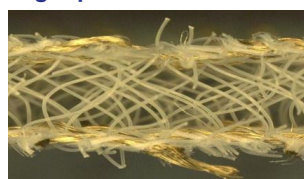
Non-conductive pile thread area made of polyester monofilament
